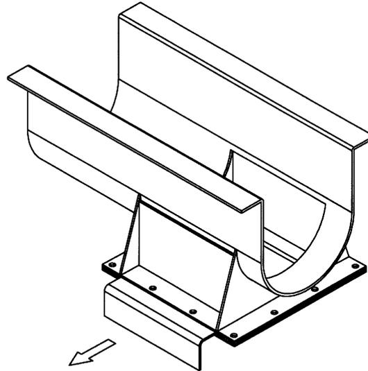
INSTALLED SLIDE VALVE WITH LONGITUDINAL OPENING TOWARDS THE CONVEYOR
